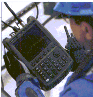
2. To enhance the field capabilities of RF test and measurement equipment, spectrum and signal-analyzer functions are built into the latest portable and rugged models. (Courtesy of Agilent Technologies)
